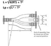
constant. A variable radius traveling loop accommodates motion by varying the bend radius of the hose assembly. Both types of traveling loops can be installed to absorb either horizontal or vertical movement. The constant radius traveling loop provides for greater movement while the variable radius traveling loop requires less installation space.
