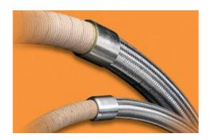
Constructed using a helical tape wrapped PTFE with a glass fibre overlay, overbraided with 304 AISI 304/S15 stainless steel. Also available with a carbon liner.
